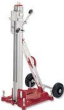
Fitted with four carriage guide rollers, a carriage brake, a "vacuum clamp" base, a set of wheels and a quick release plate . **Aluminium column** for guaranteed strength and corrosion resistance. **Drilling stroke:** 700 mm. **Angle of inclination:** 0 - 45°.
