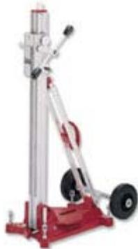
Fitted with four carriage guide rollers, a carriage brake, a "vacuum clamp" base, a set of wheels and a quick release plate. **Aluminium column** for guaranteed strength and corrosion resistance. **Drilling stroke:** 600 mm. **Angle of inclination:** 0 - 45°.
